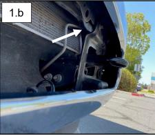
1. Using A 13mm socket, remove the 2x bolts mounting the bumper supports.
